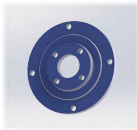
Fig. 3. 3 Attachment for Dremel Drill to be attached, a) Bottom view of Part 1, b) Side view of Part 1 with Steel blocks (c) Side view of Part 1 without Steel blocks inserted d) Drill attached to the Sawyer Robot Arm
