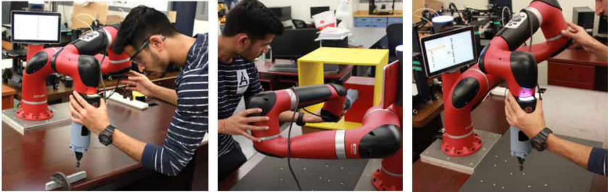
Fig. 3. 5 Kinesthetically teaching different positions
