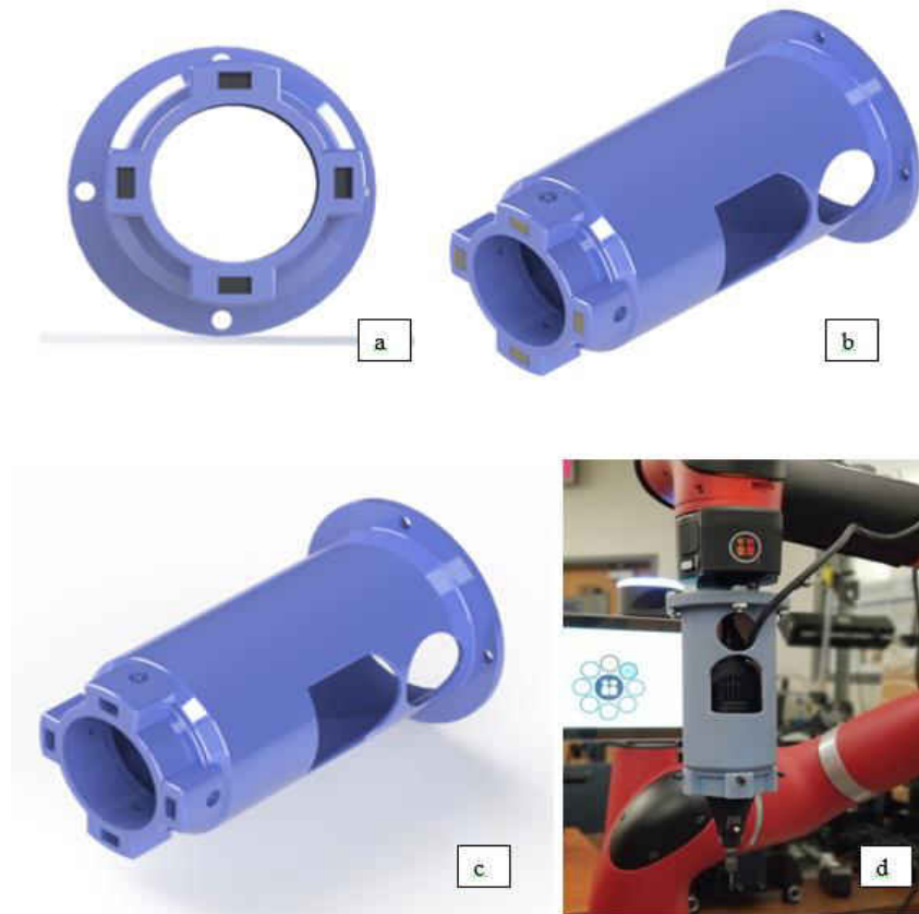
Fig. 3. 3 Attachment for Dremel Drill to be attached, a) Bottom view of Part 1, b) Side view of Part 1 with Steel blocks (c) Side view of Part 1 without Steel blocks inserted d) Drill attached to the Sawyer Robot Arm
